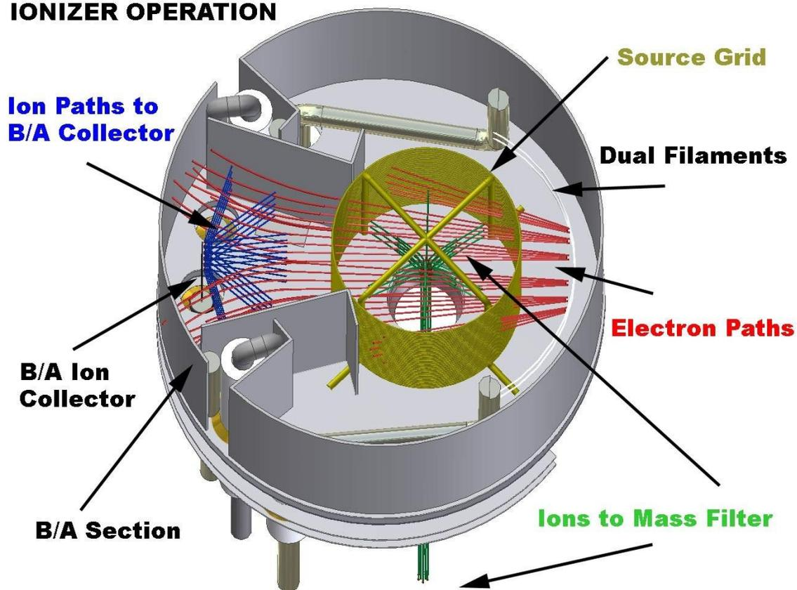
Figure 1 Extorr XT Series Ionizer
