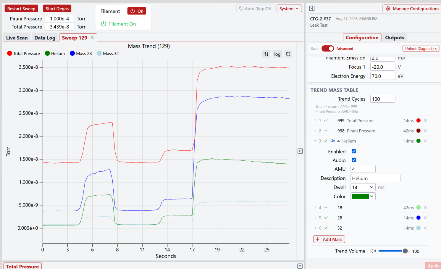
Trend Mode Pressure vs. Time with Leak Detect Audio On
