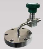
**Description:** XT Series Single Valve Sampling Inlet has one metal sealed on-off valve mounted on a DN 40 CF, 2 <sup>3</sup>/<sub>4</sub> inch ConFlat (CF) flange with a Swagelok type nut and ferrule fitting for connecting the capillary tubing. The inlet assembly is made from 304 stainless steel. Stainless steel mounting hardware, and a 2 <sup>3</sup>/<sub>4</sub> inch CF copper gasket.
