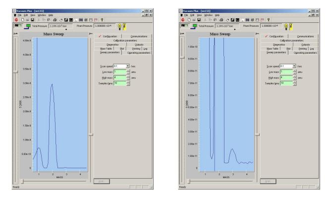
The spectra above from an ion pumped system shows data for masses 1, 2, and 3 at two intensity scale settings.
